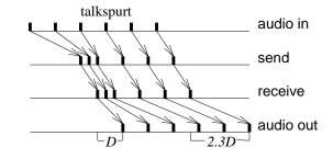
Figure 8: Effect of packet caching on playout delay
