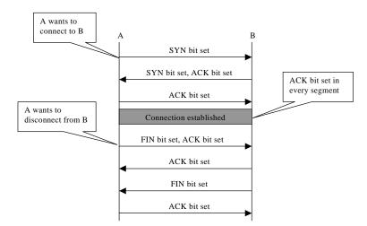
Figure 14. Setup and tear down of a TCP connection
