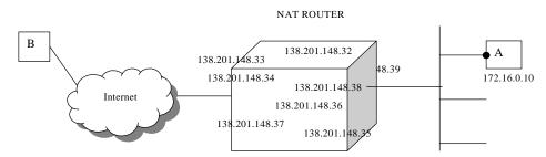
Figure 25. A NAT router with a pool of addresses
