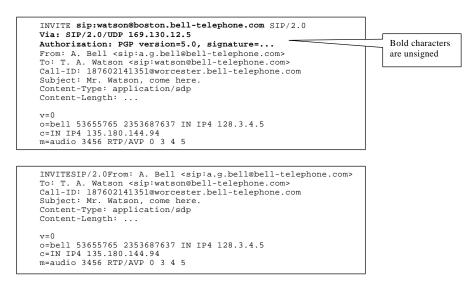
Figure 29. Upper - the SIP request that is to be sent. Lower - the signed parts of the message
