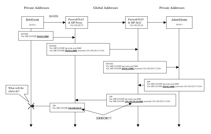
Figure 32. Receiver tagged Via field
