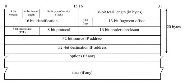
Figure 5. The IPv4 header
