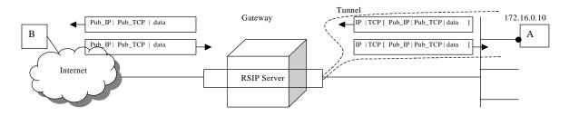
Figure 37. Tunneling with RSIP
