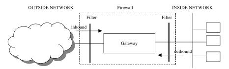
Figure 13. The principles of a firewall
