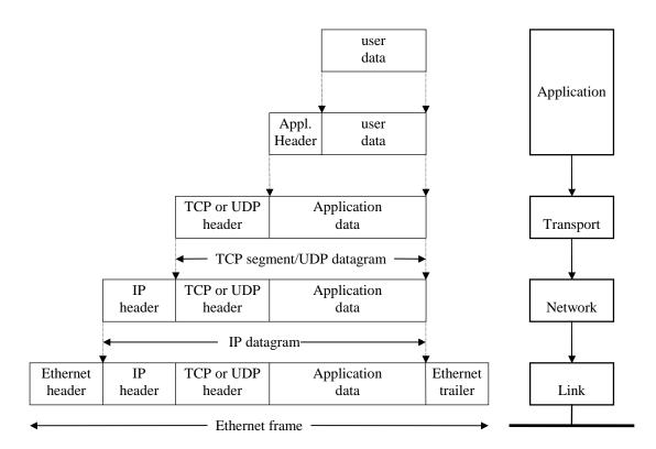
Figure 2. Encapsulation and layer distribution
