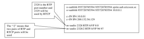
Figure 31. Examples of origin-, connection-, and media-fields
