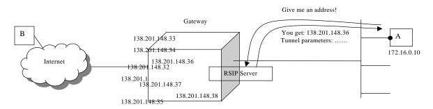
Figure 36. Request to an RSIP server for a public address
