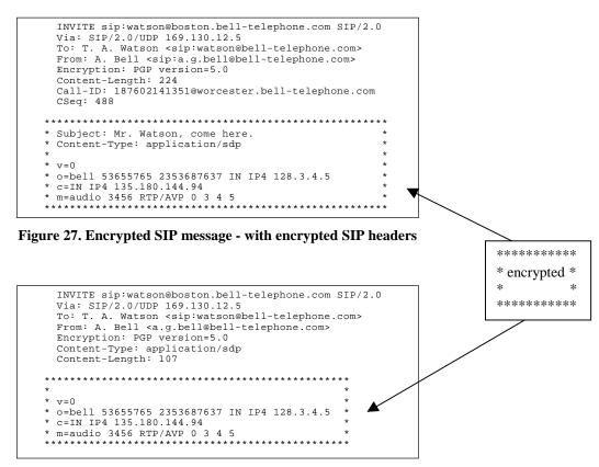
Figure 28. Encrypted SIP message - with no encrypted SIP headers
