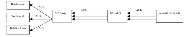
Figure 35. Forking Proxy - ACK message
