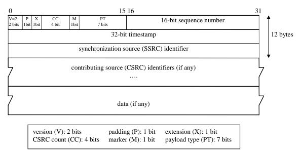
Figure 1. The RTP header
