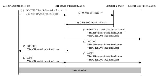
Figure 11. SIP Server in proxy mode
