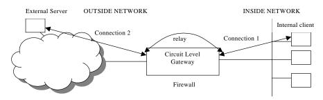
Figure 16. Circuit Level Gateway
